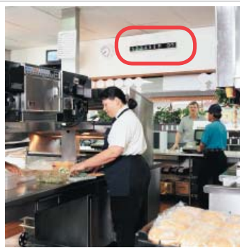
Number Panel visible to entire cooking staff, displays production level.
